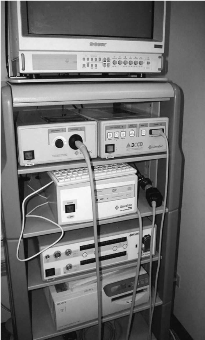
FIGURE 9.20. The arthroscopic stack of equipment that is necessary to perform arthroscopic surgery, including the fluid pump.
