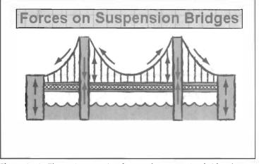
**Figure 25-2.** The action-reaction forces of a suspension bridge that supports the weight of the roadway.
