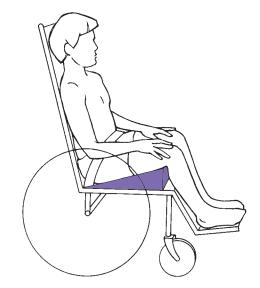
**FIGURE 7.3** Child is supported in a wheelchair with a tall back and a seat wedge to maintain hip flexion. The back may be designed to either recline or tilt in space to accommodate fatigue in the child.
