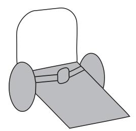
**FIGURE 12.11** The pre-wheelchair device allows the child to be mobile on the floor and teaches the use of the upper extremities for propelling the wheelchair.
