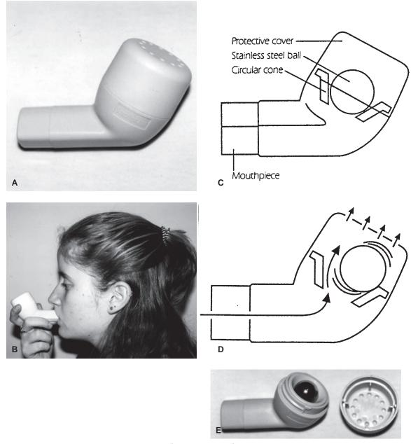
**FIGURE 20.10** (A) Flutter device (VarioRaw SA, distributed by Scandipharm, Inc., Birmingham, AL). (B) Flutter device in use (compliments of A. Tecklin). (C) Cross section of Flutter device. (D) Cross section of Flutter device with representation of oscillating ball. (E) Flutter device with oscillating ball.
