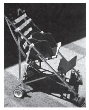
**FIGURE 12.1** Umbrella-type stroller with a tri-wall insert and foot support.
