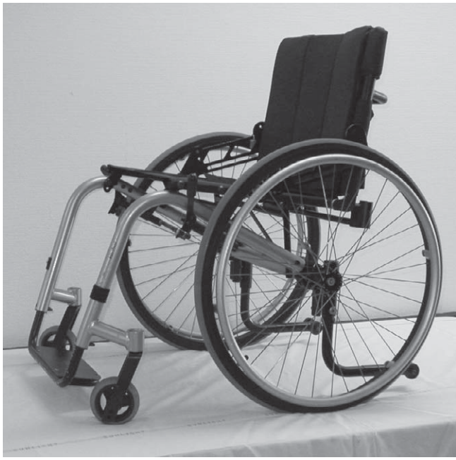
Figure 11.2 Example of high performance rigid frame wheelchair.
