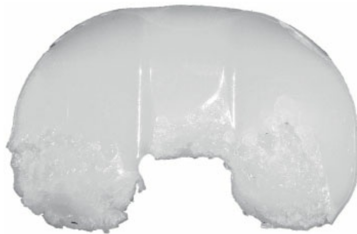
FIG. 16-13 Tibial polyethylene plateau with delamination damage—probably due to misalignment.
