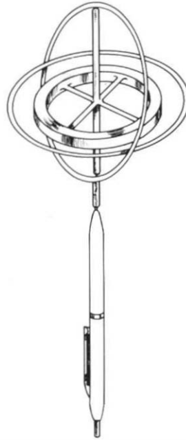
FIGURE 9-2 Angular acceleration. A gyroscope balances on the tip of the pen because of the high rotatory speed of its wheel. If it tilts to the side, an angular acceleration and a moment develop, restoring it back to its original position.
