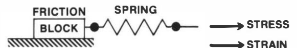
FIGURE 9-46 Plasticity. A block being pulled by a force via a spring is used to explain the elastic and plastic behaviors. AB = elastic loading (spring); BC = plastic deformation (friction); CD = elastic unloading (spring); AD = permanent deformation (friction); DCE = reloading cycle; DCE \equiv ABC.
