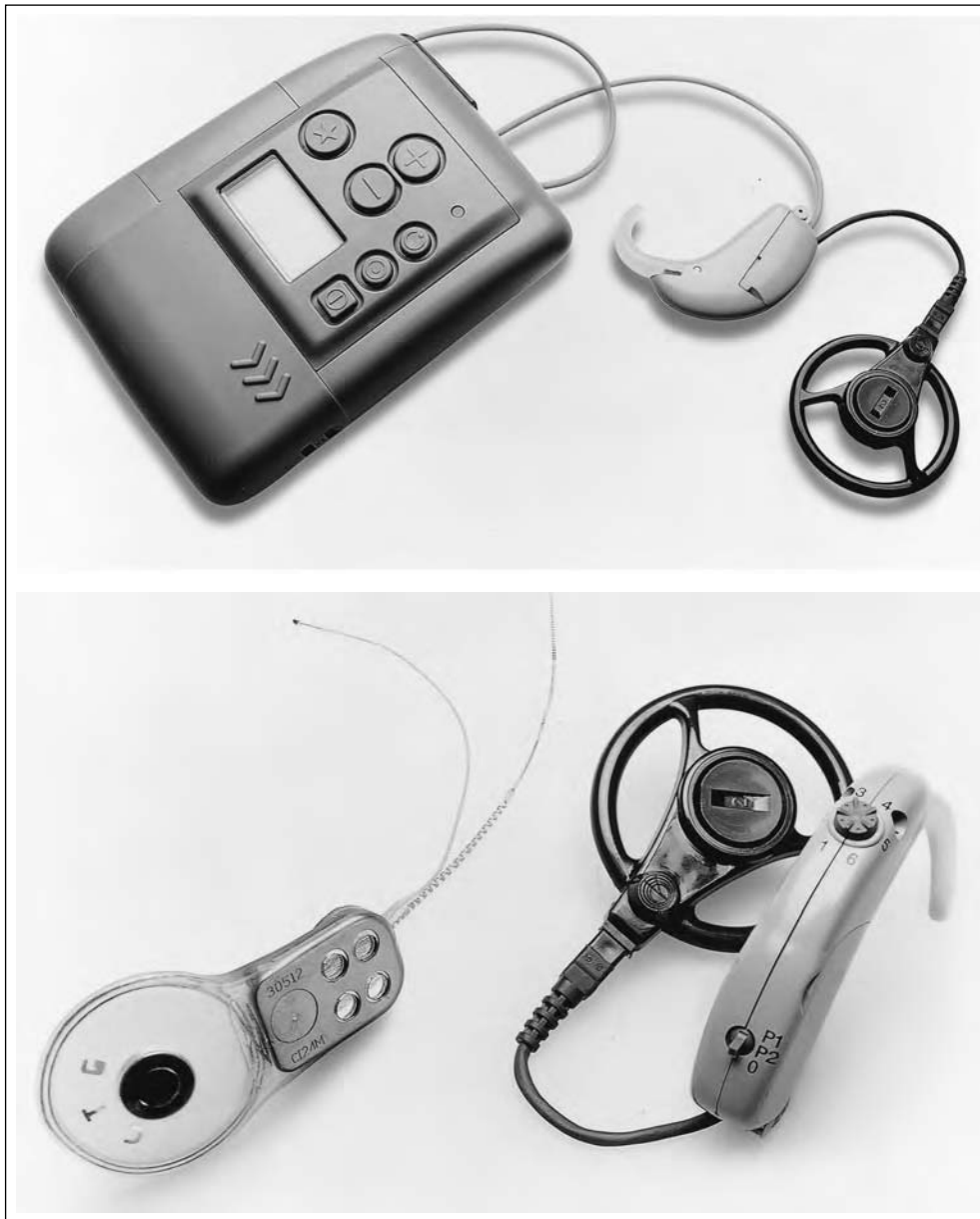
Figure 10.8 (A) A multichannel cochlear implant processor, microphone, and magnet coil. (B) Cochlear implant internal device electrode array and ear-level cochlear implant. (Photographs courtesy of Cochlear Corporation.)
