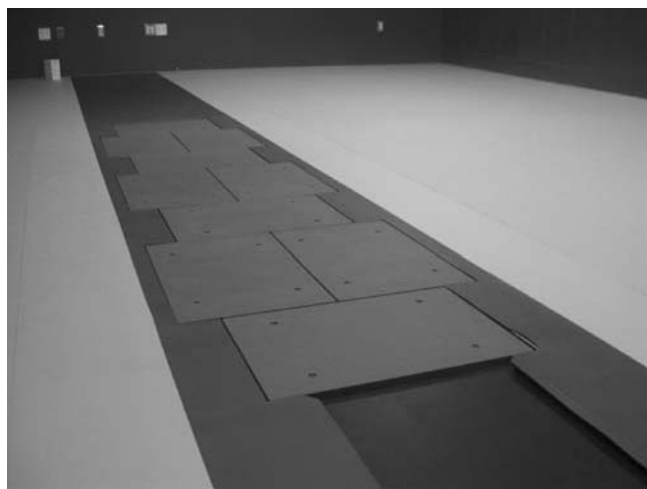
FIGURE 5.7 Large 10-platform array of 60 cm × 40 cm force platforms used in The Center for Gait and Movement Analysis at Children's Hospital Colorado in Aurora, Colorado. The "hopscotch" pattern of the platform array permits the recording of several individual foot strikes from both feet in a single walking pass. For illustration purposes, each platform is shown without its protective floor covering, which caused the platforms to blend into the surrounding walkway when applied.
