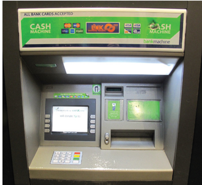
Figure 6.1 Everyday example of human factors engineering – a cash machine, or ATM. Cash machines around the world have the same design – from the arrangement of the numbers on the keypad to the fact that the machine beeps and flashes to remind you to take your card before it dispenses your cash. This is an example of human factors engineering, design that takes into account that ‘to err is human’. How many of us would walk off leaving our cards behind if cashpoint machines did not operate this way?
